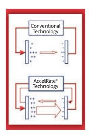
intervals discharge cycles into the charging profile. This homogenizes the ion field around the plates, promoting a far better distribution of the active ions over the entire charging area.
